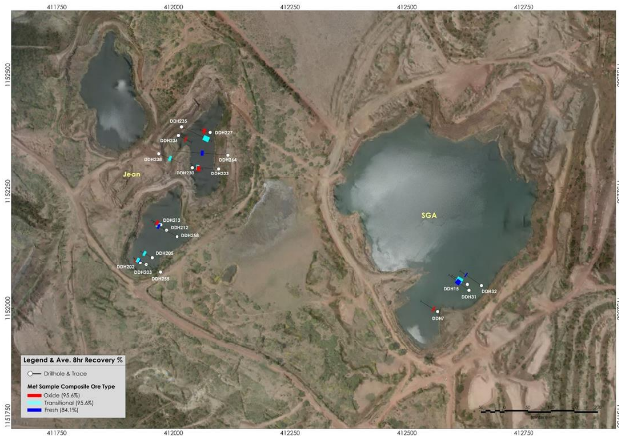
Figure 13.2 Drillhole locations and sample intervals of the Lakefield bulk composite metallurgical samples
