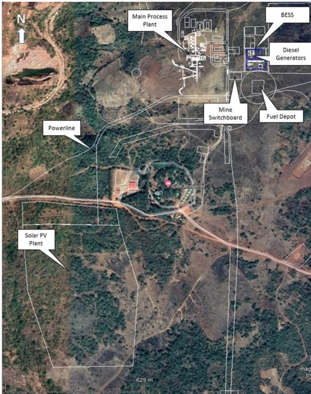
Figure 18.4 General infrastructure layout for Project power facility
