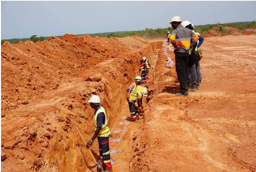
Figure 16-4 Ore control - Trench sampling
