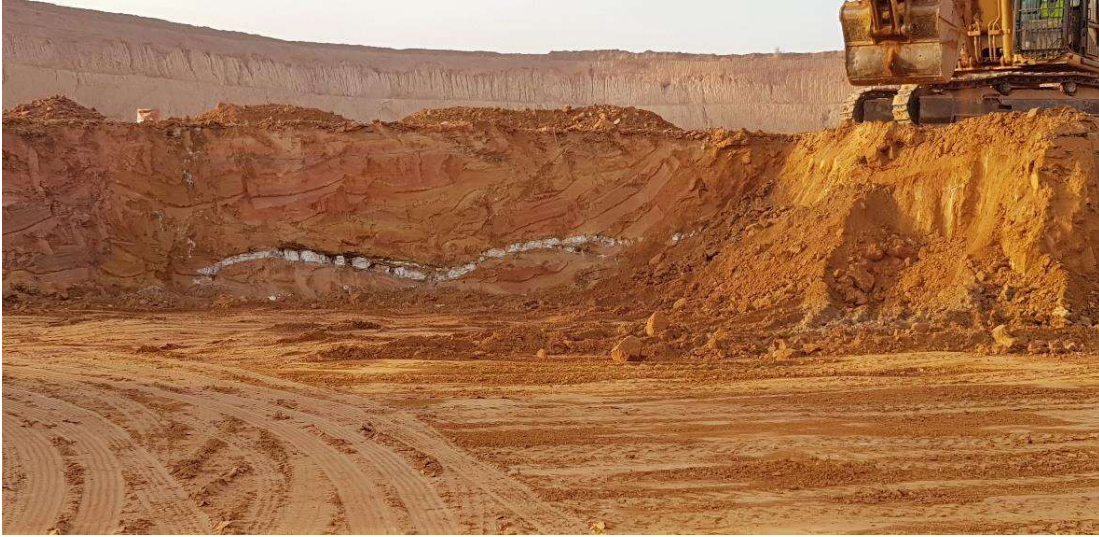
Figure 7-17 Undulating flat veins dipping 25-30° SSW to SSE, Central Domain.
