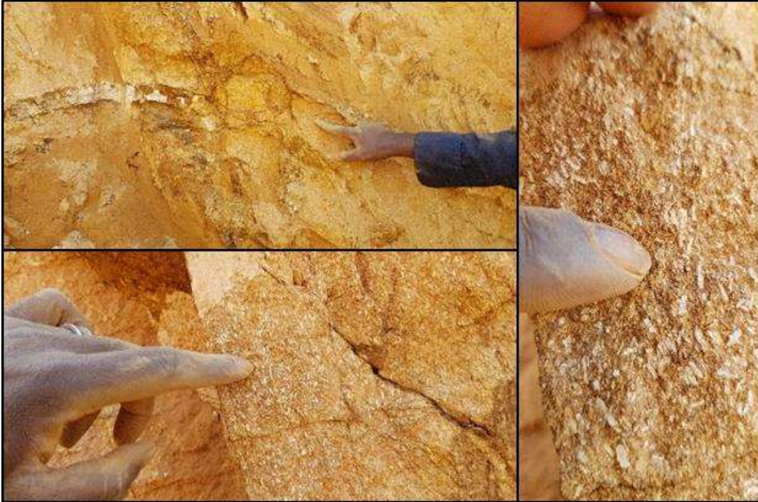
Figure 7-10 Porphyritic gabbroic dyke displaying kaolinized tabular
