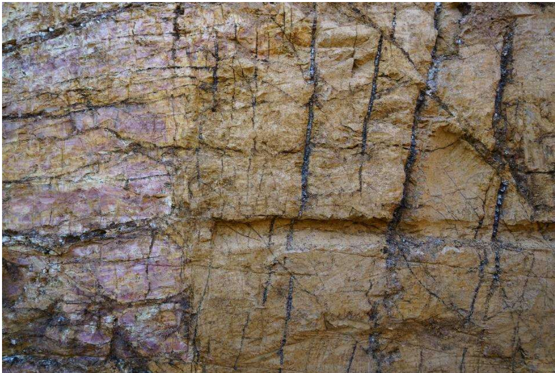
Figure 7-9 Gabbroic intrusive (A) in contact with turbidite (B) (hornfelsed flysch).
