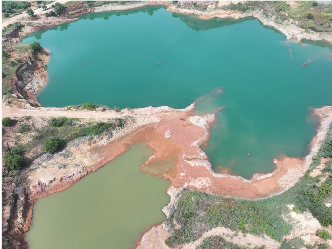
Figure 3: SGA pit dewatering progress with an approximated 9m drop.
