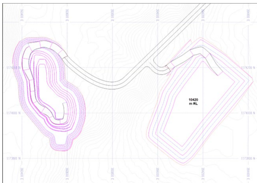
Figure 16.16: BC Waste Rock Dump Layout
