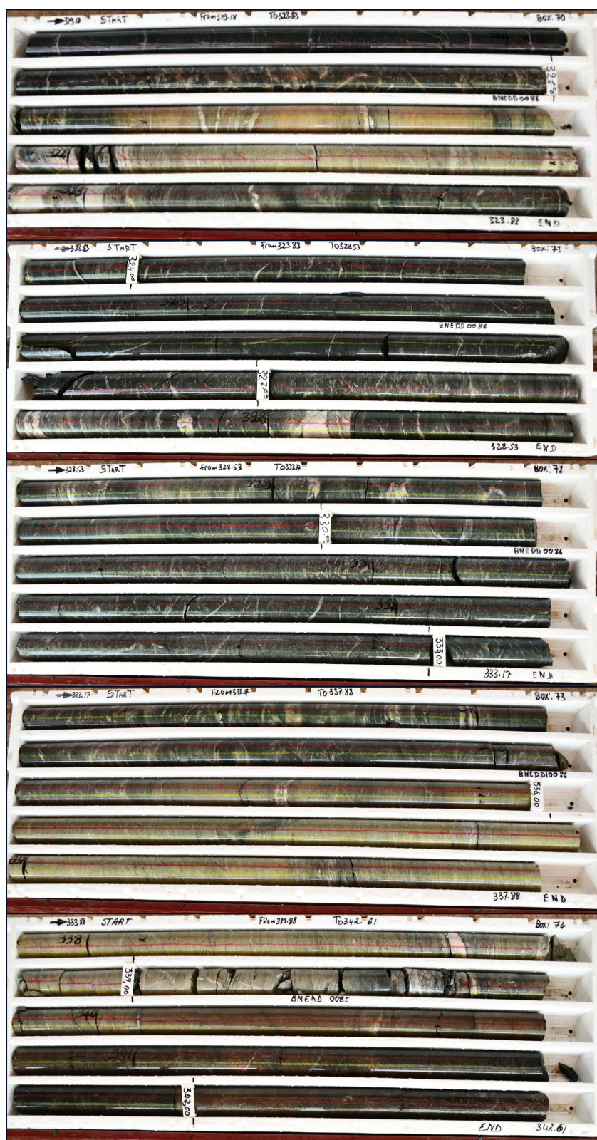
Figure 7.13: BNEDD0086 Main Shear 320.0-340.1m, 20.1m @ 0.48g/t
