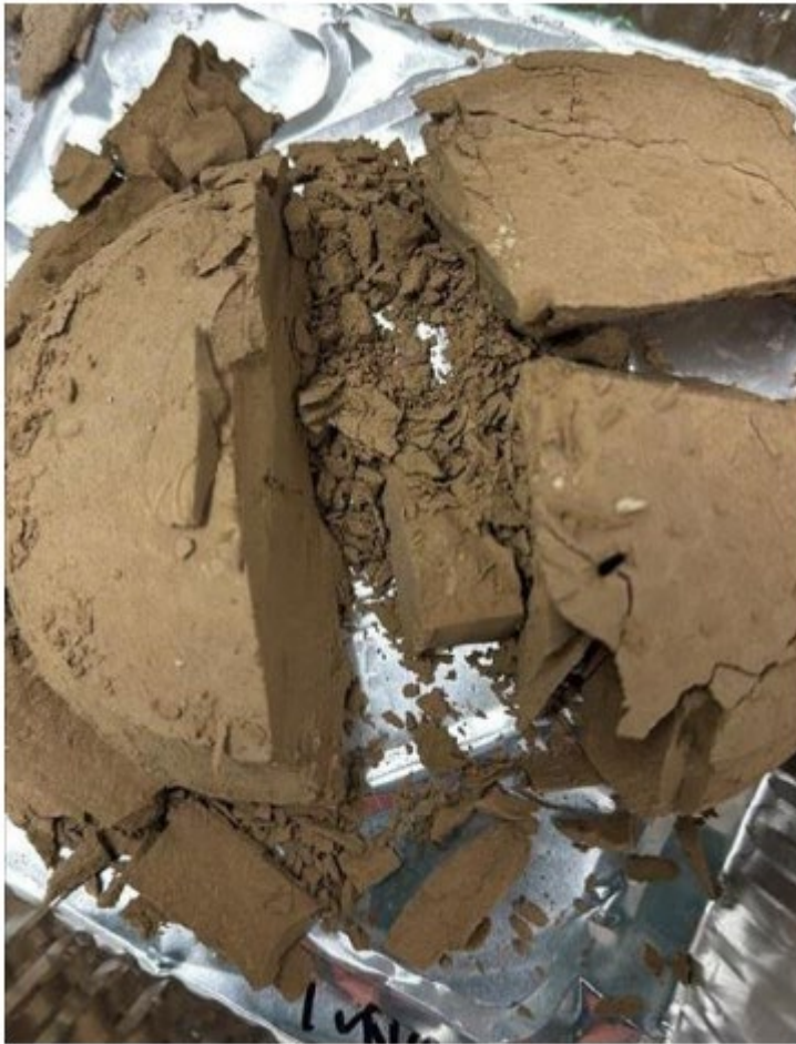
Figure 13.24: 50% Saprolite Sample from 40mm Chamber @15.9% Moisture
