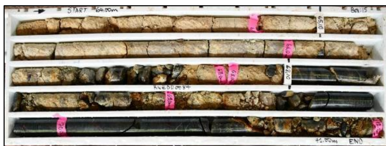
Figure 7.6: BNEDD0087 Contact Between Saprolite Zone (upper) and Saprock Zone (Lower)
