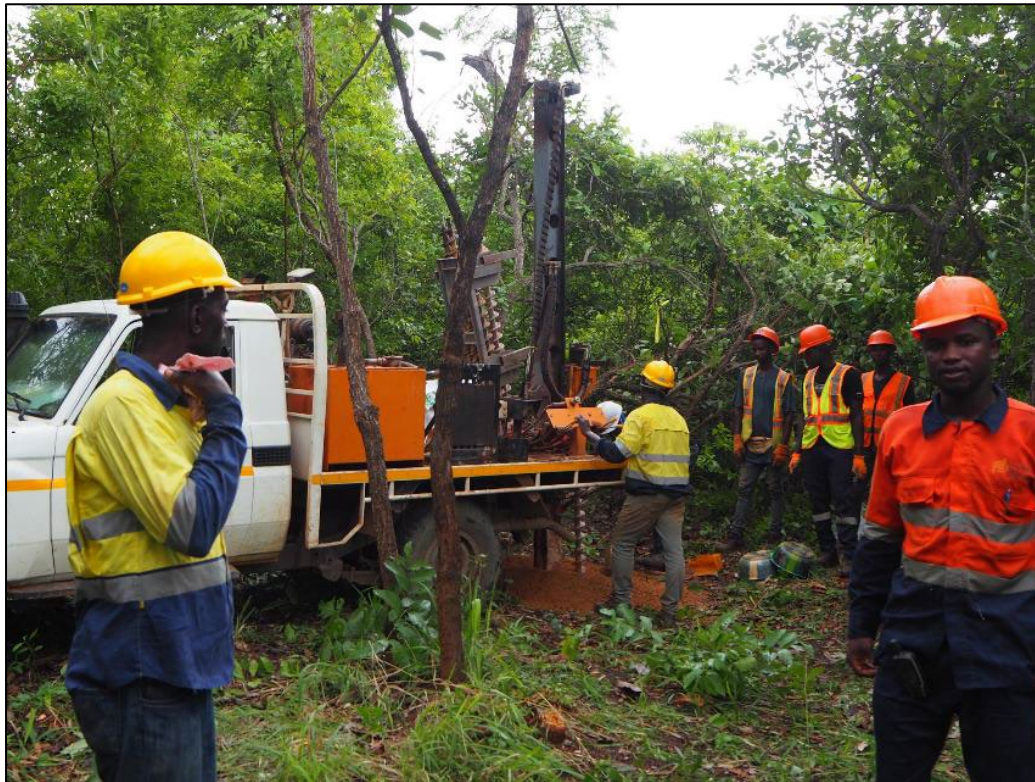
Figure 10.2: Auger Drill Rig (PDI 2024)
